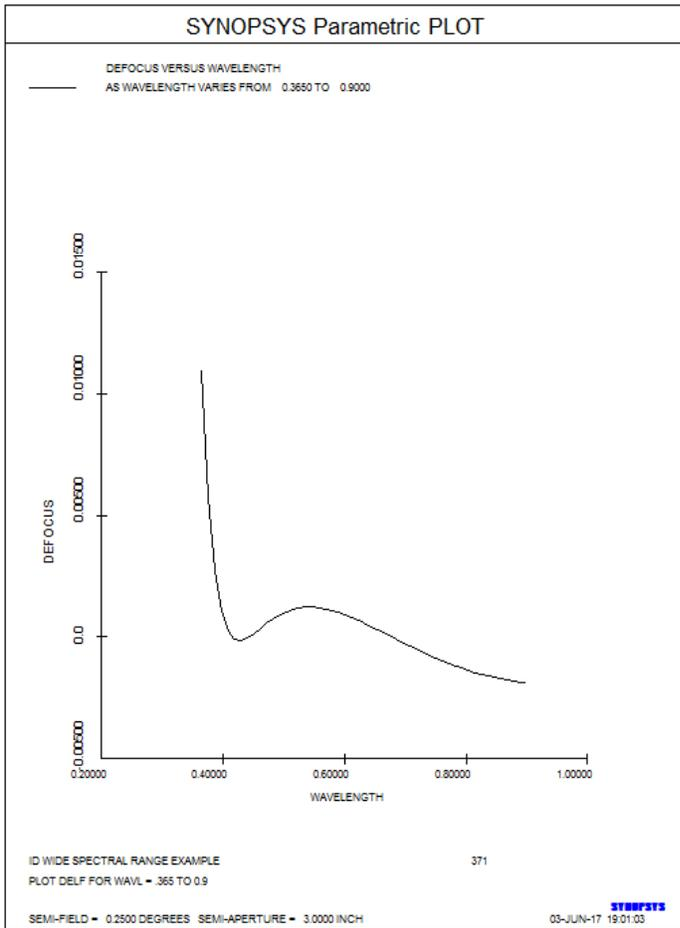
Well, it's corrected at three wavelengths for sure – but we are aiming for four. How come the curve doesn't go up again at the right end – as a true superachromat would? Simple. As usual, the program is balancing everything in the merit function, not just axial color, and a small amount of sphero-chromatism makes it depart slightly. Still, this is a great lens!
