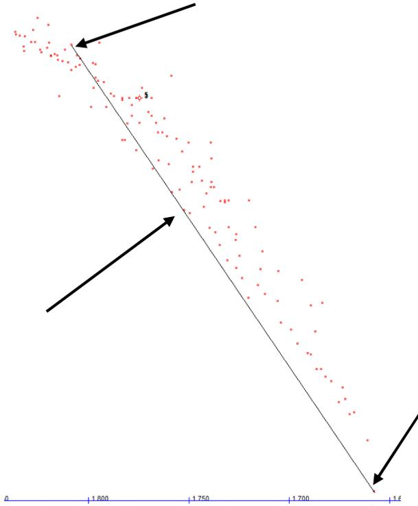
We have three potential glasses for our superachromat. They are types S-PHM52, S-NPH5, and S-TIL27. You can also display the relative cost and other properties, to help you select three acceptable glasses. Then you insert those three glasses into the lens and optimize. If that does not yield a satisfactory lens, you select a different three according to the same procedure. This process is rather tedious but often works quite well.
