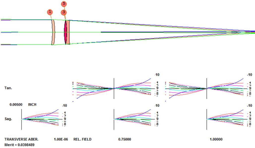
How good is this state of correction? We can ask AI to show us the defocus over wavelength – but that would be unwise at the moment. This lens has a curvature solve, and at each wavelength the program would recalculate it. (We surely don't want that to happen!) So instead, we make a second MACro, as follows:
